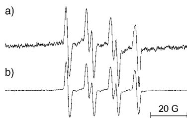
Figure 1. EPR spectra of DMPO–SC 4 H 9 spin adducts a) trapped during the exchange reaction of triphenylphosphane-protected Au nanoparticles with butanethiol and b) prepared by the oxidation of butanethiol with PbO 2 in the presence of DMPO.
